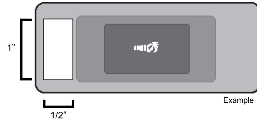
Dimmer switch panel
